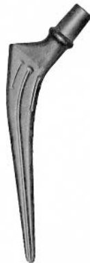
Fig. 1.4 Hip endoprosthesis stem, injection molded, chopped long fiber reinforced PEEK, fiber volume content 50% [M. Semadeni, Ph.D. Thesis, ETH Zurich, 1999].
