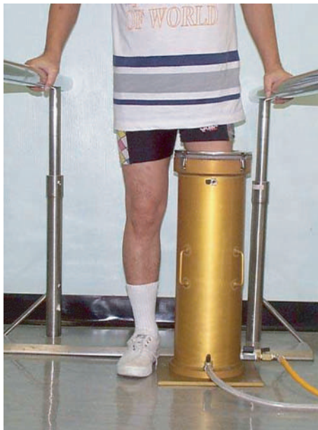
Fig. 7.21 A hydraulic casting system [Huang and Ramakrishna, 1999].
