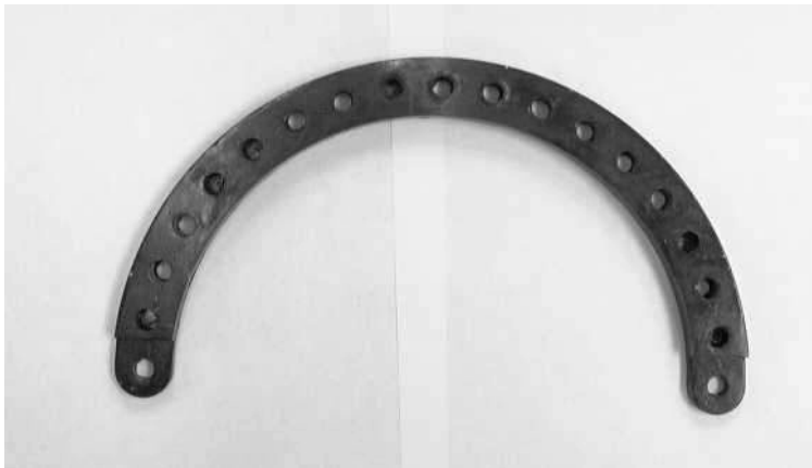
Fig. 7.27 A half-ring of an external fixator made from chopped carbon fibers and thermoplastic PEEK matrix through a hot press.
