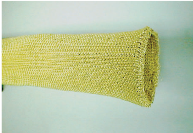
Fig. 7.22 A sleeve form of rib knit Kevlar 49 fiber fabric used in this study.
