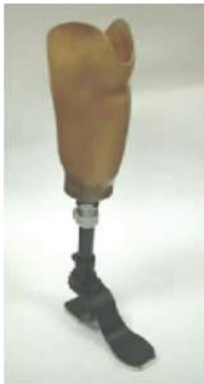
Fig. 7.23 A prototype direct socket using two layers of Kevlar 49 fiber rib knitted fabrics and a UV activated resin [Huang and Ramakrishna, 1999].
